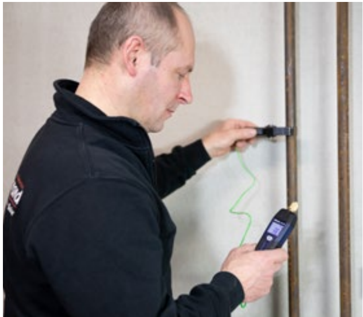
The temperature measuring clamp can be used to determine the pipe temperature.
