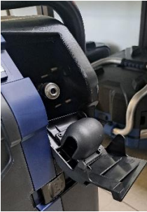
Fig. 23: The transport lock can be stored in the camera flap
