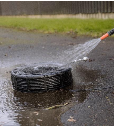
Fig. 91: Hosing off the reel and rod
