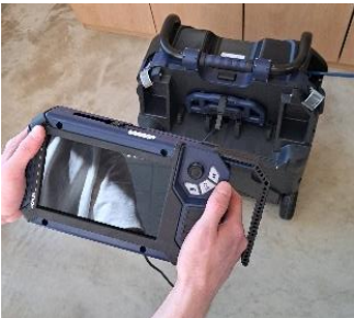
Fig. 28: Monitor pulled out of the trolley holder
