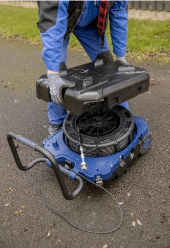
Fig. 98: Attaching the lower shell
