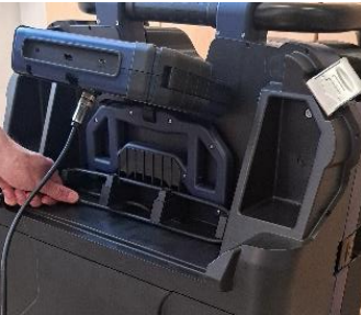
Fig. 99: Wrap the monitor cable around the cable domes
