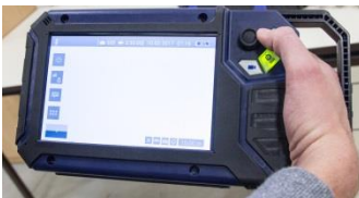
Fig. 32: When the handle is extended, the monitor can be held and operated with one hand.
