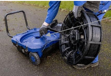
Fig. 94: Pull the connection cable through the opening of the reel holder
