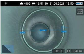
Fig. 63: Display of the distance between two measuring points
