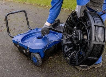
Fig. 16: Pull the connection cable through the opening in the reel holder.
