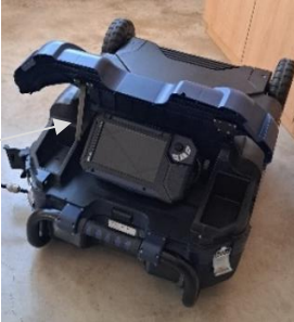
Fig. 34: Wöhler VIS 750 HD inspection camera in horizontal position with glare shield
