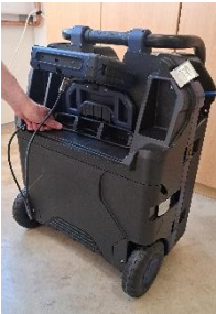
Fig. 31: Roll up the connection cable before pushing the monitor back in.
