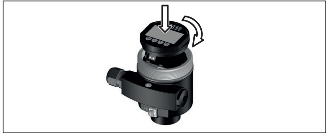
Fig. 26: Installing the display and adjustment module in the electronics compartment of the single chamber housing
