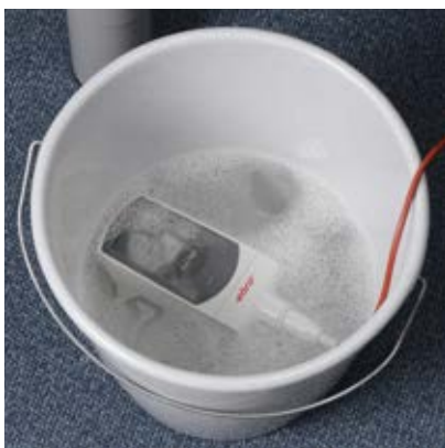
TF 410 - still working, thanks to IP67
