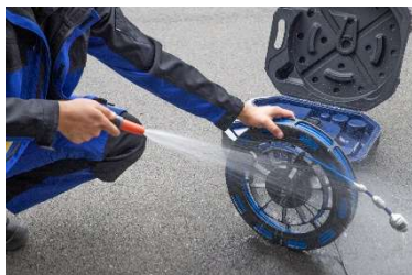
Fig.42: Hosing down the reel and rod
