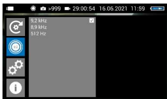
Fig.29: Location transmitter with 9.2 kHz transmission frequency selected
