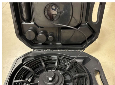
Fig.45 : Incorrect: Camera cable not pulled taut
