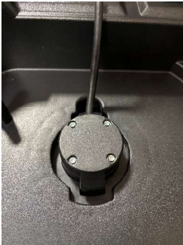
Fig.44: Insert the camera cable into the upper shell and pull it taut carefully
